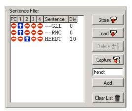
If for instance the GGA and GLL sentences have to be blocked, simply click on the pass signs of both sentences, to change them into a block sign. Pressing the Store button sends the list to the multiplexer. Now the filter is operational.
