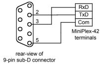
The RS-232 interface behaves in exactly the same way as the Bluetooth interface. All received NMEA data is available on both the RS-232 and the Bluetooth interface. If data is sent to the RS-232 interface in Hub-mode, it will not only be sent to the NMEA Out2 port, but also to the Bluetooth interface.
