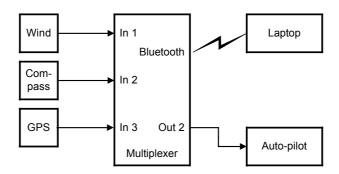
When the laptop is on board, it will receive all information from the instruments and the running navigation software is able to calculate the course to steer and drive the autopilot accordingly. Because the laptop is sending NMEA data, the multiplexer is in server mode and the autopilot will therefore receive information from the laptop only.
